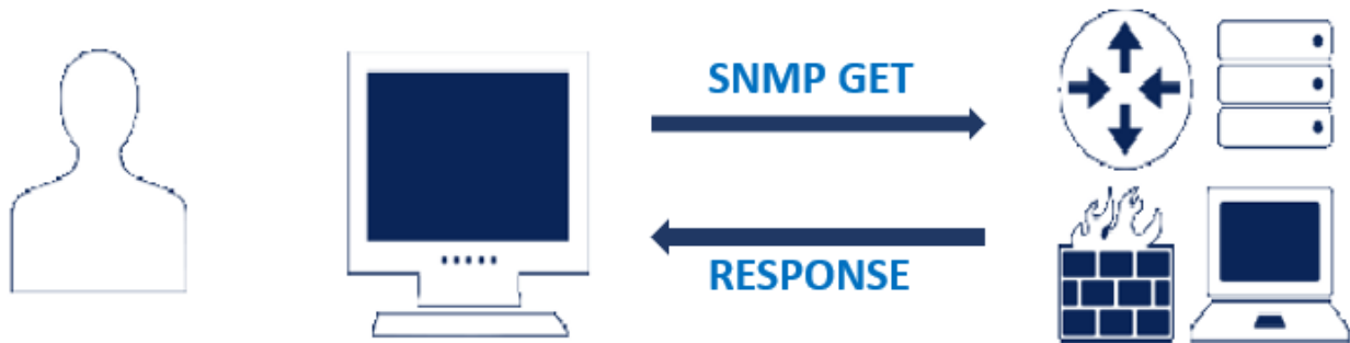
Figure 15: SNMP message flow
